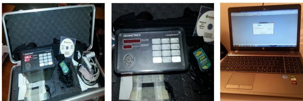
Figure 8. The appearance of the proton-type magnetometer G-856, manufactured in America.
