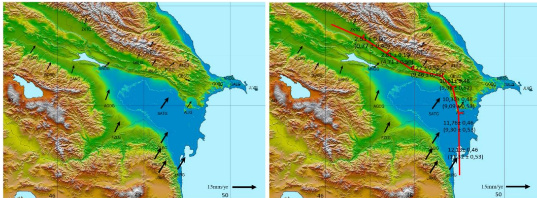
Fig. 3. Horizontal velocity vector map for 2014-2022 and fault velocities (mm/yr) obtained from the block model.
