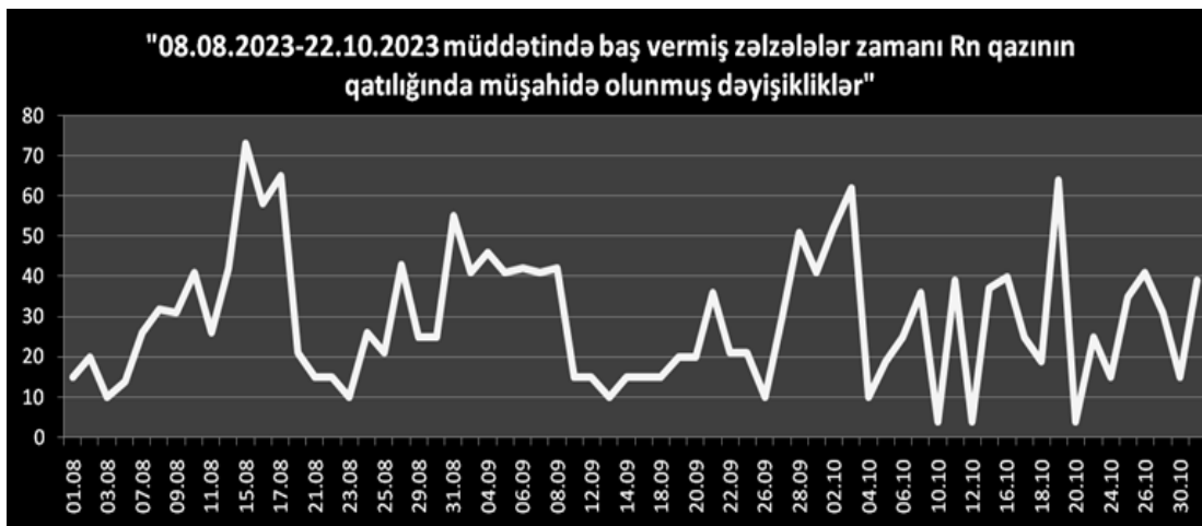
Figure 6. Changes observed in the concentration of Rn gas during the earthquakes that occurred between 08.08.23 and 22.10.23
