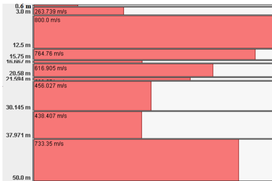
Fig. 6. 1-dimensional velocity cross-section of a transverse wave along a seismic profile at a construction site in Nizami district
